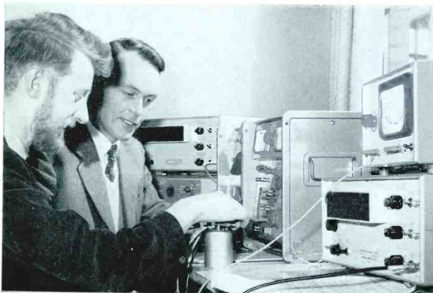
Mr. A. Spencer, of our U.S.A. Office, and Mr. T. Clarke, Midland Area representative, testing coil characteristics with a Circuit Magnification Meter type TF 1245 (centre) and Sensitive Valve Voltmeter type TF 2600 (top right)
